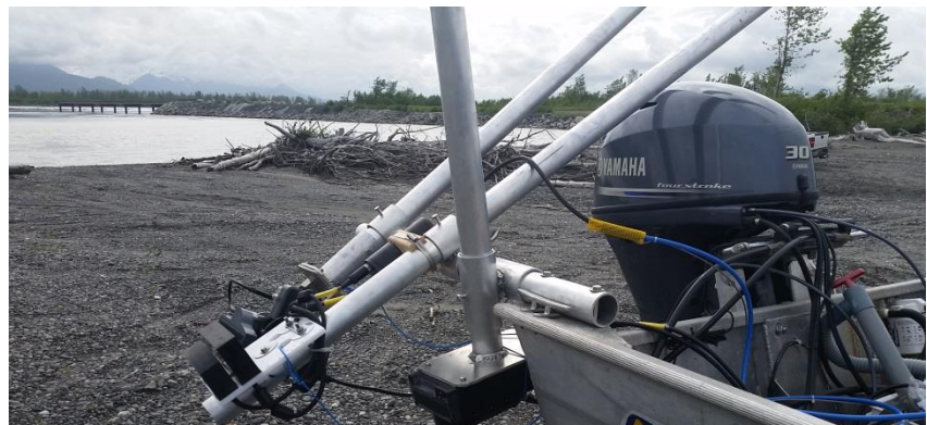
Figure 2: Skiff-mounted sonars prior to the first in-river test, June 12th 2015. Sonar systems from left to right are the Imagenex 965, PicoFLS, and Gemini.
